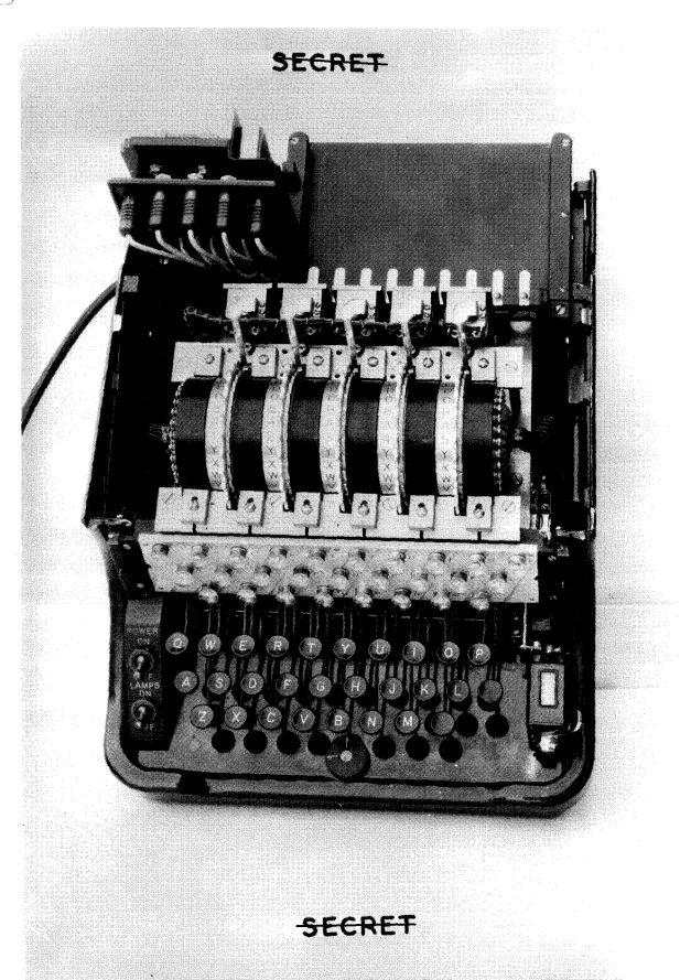
Fig. 6 - Converter M-134-T2, Plan View, Covers Removed
