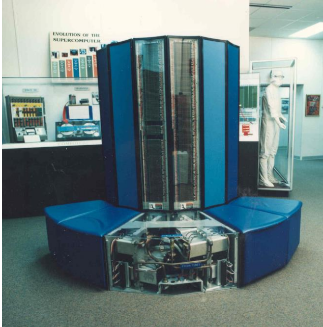
The Cray 1 on display in the National Cryptologic Museum. Notice the "seats," which circulated the coolant.
