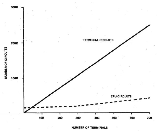
Fig. 4—Circuit Distribution in a Teleprocessing System
