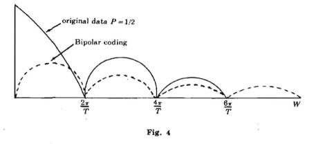
It is evident that the predominance of low frequency power does not exist for the bipolar coded version of the data for  $\Delta = T p = 1/2$ .
