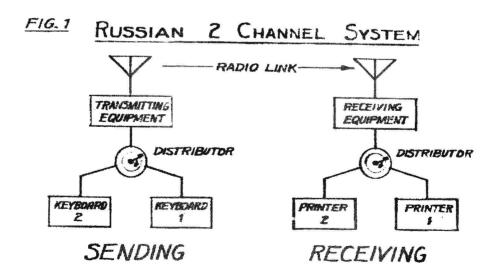
Schematic drawing of Baudot sending and receiving system
