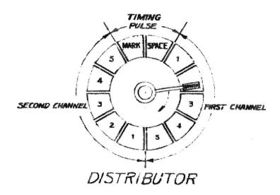
Schematic drawing of the distributor system
