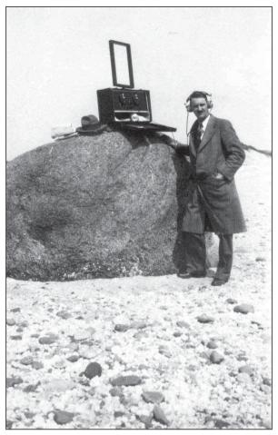
Direction finder model in use through 1930. Then a smaller, more modern apparatus was built that could be mounted in an automobile. (Photo from *Rum War: The U.S. Coast Guard and Prohibition* by Donald L. Canney)
