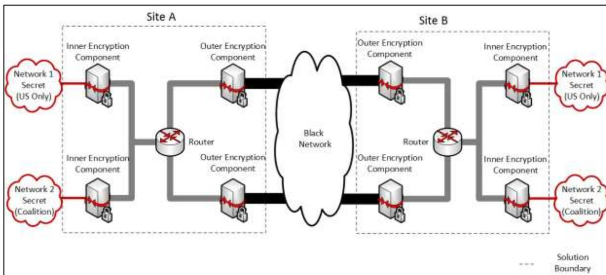
**Figure 9. MSC Solution with Redundant Outer Encryption Components**
