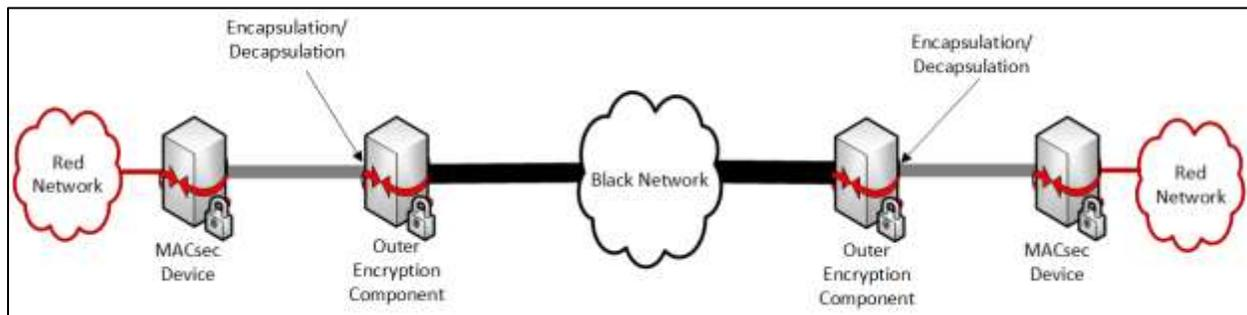
**Figure 7. Encapsulating MACsec on an Internal Interface**
