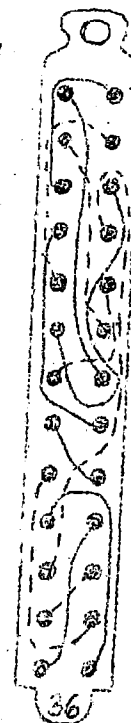
FIG. 4. SLIDE. SHOWING PRINTED CIRCUIT. (DOTTED LINES PRINTED ON REVERSE SIDE)
