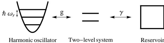
FIG. 1: This figure shows the physical system described in this article. A quantum mechanical harmonic oscillator of frequency  $\omega_r$  is coupled with a strength  $g$  to a two-level system which in turn is damped at a rate  $\gamma$  by a bath at zero temperature.
