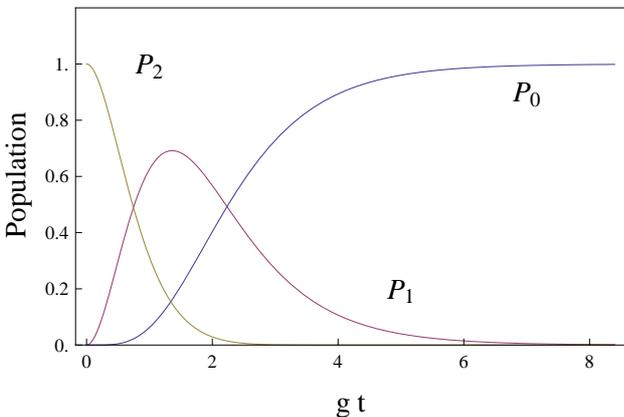
FIG. 3: This figure shows the time evolution of the populations  $P_n$  in the oscillator states  $n = 0, 1, 2$  for the case shown in Fig. 2. The initially occupied  $n = 2$  state eventually decays, the  $n = 1$  state is transiently populated, and  $n = 0$  is ultimately occupied with unit probability.
