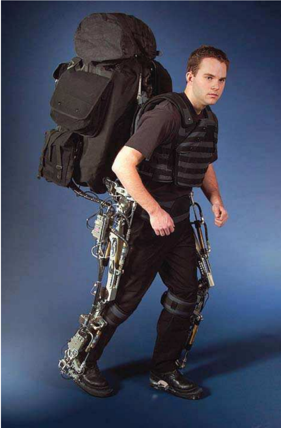
The Berkeley Lower Extremity Exoskeleton (BLEEX) helps lighten the load for the human user. Image credit: UC Berkeley
