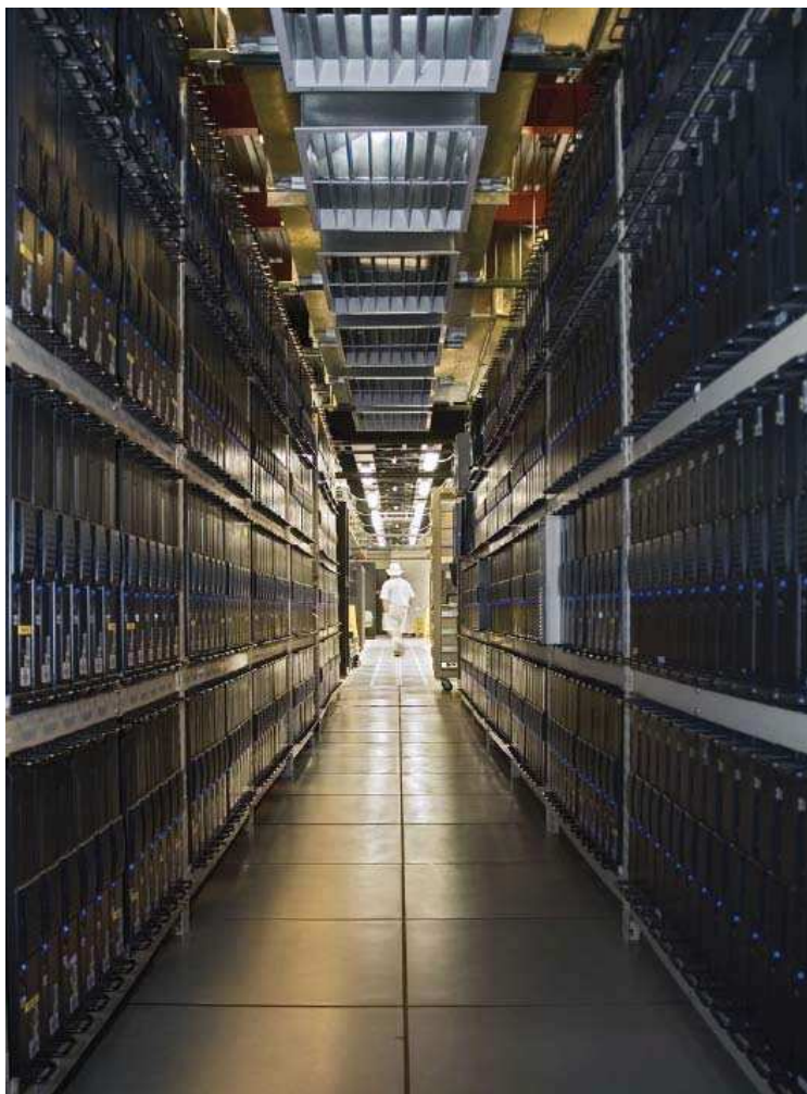
The “Kaon” virtual supercomputer in the Fermilab Lattice Computing Center runs on a cluster of 600 units connected by a high-speed network. Kaon is used to help physicists better understand particle behavior.
