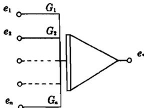
$$e = -\int_0^t (G_1 e_1 + G_2 e_2 + \dots + G_n e_n) dt$$
