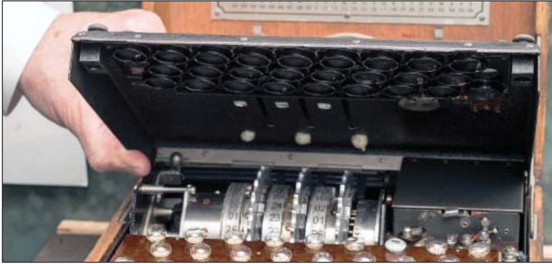
Close-up of rotors inside machine. Reflector is to the left.
