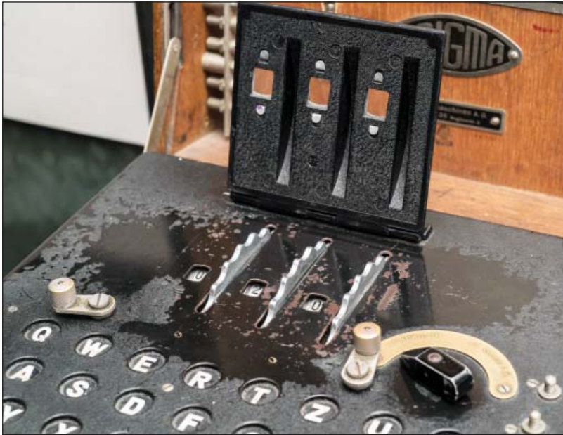
Initial rotational position of a three-rotor Enigma
