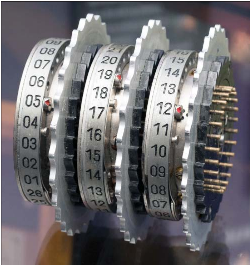
Close-up of rotor, twenty-six contact points, notch, and serrations
