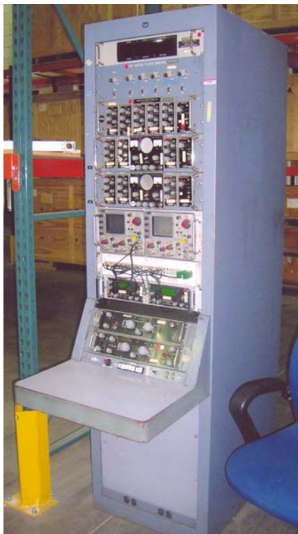
TELINT signal collection position in early 1970s
