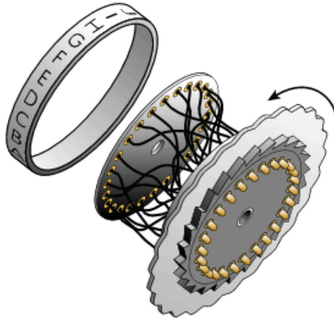
The crypto rotor wheels William Friedman envisioned for his device were flattened cylinders with an alphabet around the circumference. One face of the cylinder had twenty-six spring-loaded copper pins protruding from it; the other face had twenty-six flush copper contacts. Inside each cylinder was a wire maze connecting the electrical contacts on one side to the pins on the other.
