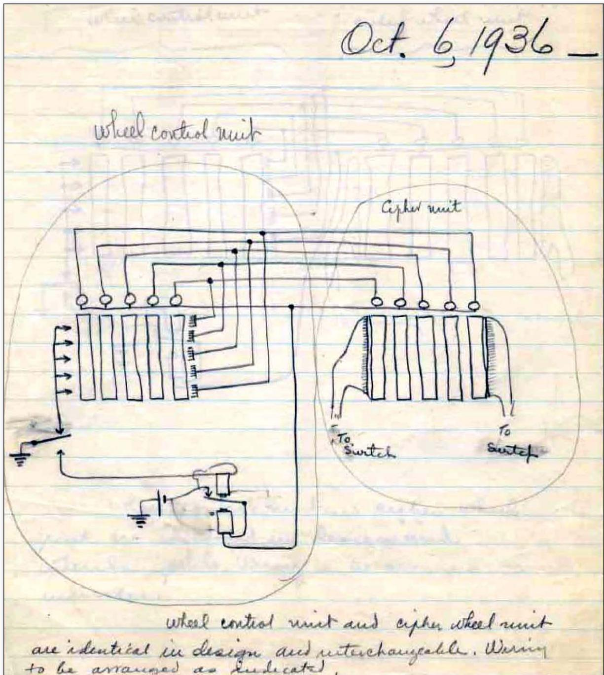
A sketch of the wheel control unit, the "control rotor bank," separate from the cipher unit, called the "cipher rotor bank." Note at bottom reads, "Wheel control unit and cipher wheel unit are identical in design and interchangeable. Wiring to be arranged as indicated."
