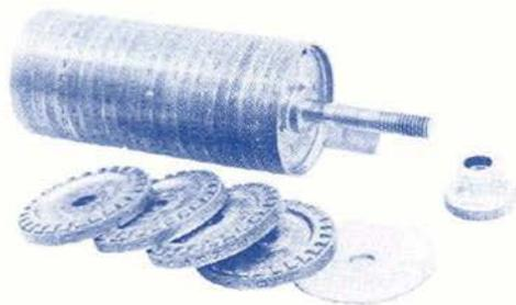
**U.S. Army cipher device M-94, developed in the 1920s. The M-94 was virtually identical in principle to Jefferson's cipher wheel.**
