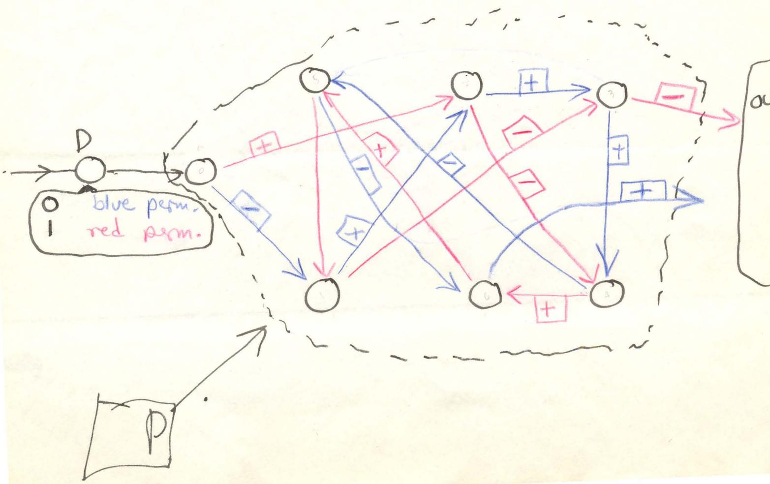
The circles represent places where a digit can be stored. During each cycle either the red permutation of digits or the blue takes place. This is decided by the digit in D at the beginning of the cycle. The D digit moves to the first ~~circle~~ storage place in P during the cycle after it has determined the choice of the permutation.
