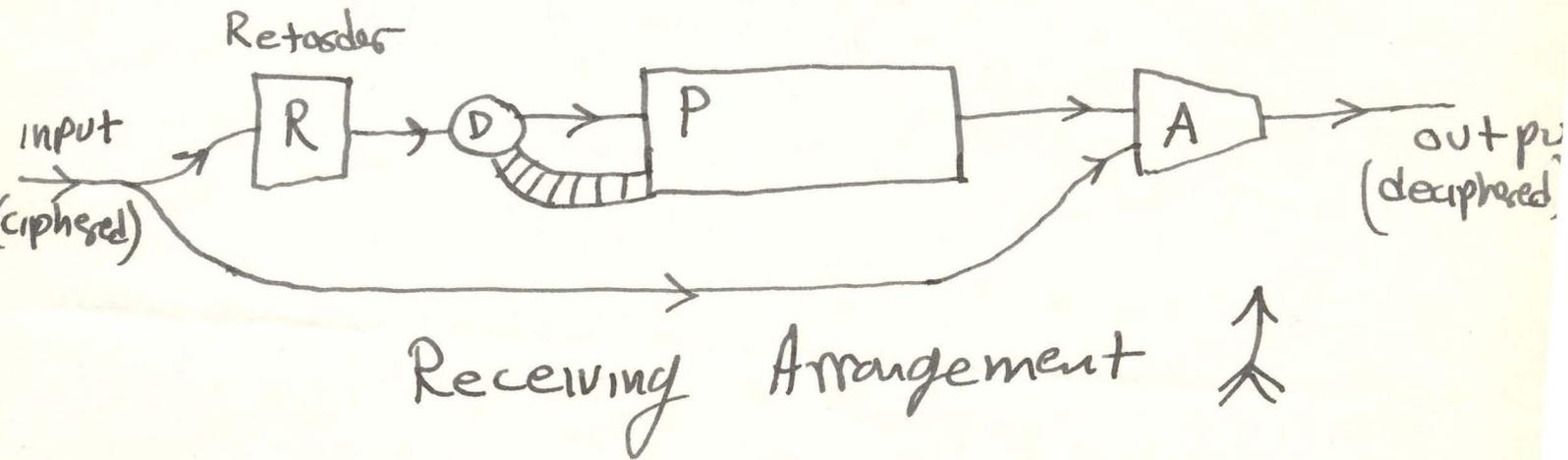
In the receiving arrangement the same components are used except for the addition of the retarder, which is a one-unit delay. The messages are to be sequences of binary digits (numbers mod 2). The machines work on a cycling basis, performing certain operations
