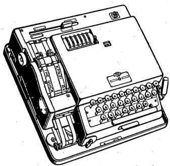
FIG. 11.—THE CRYPTODEVICE OF FIG. 9 EQUIPPED WITH A KEYBOARD AND DRIVEN BY AN ELECTRIC MOTOR. THE TWO MACHINES ARE CRYPTOGRAPHICALLY INTERCOMMUNICABLE. THE OPERATING LEVER AT RIGHT IS USED IN CASE OF POWER FAILURE
