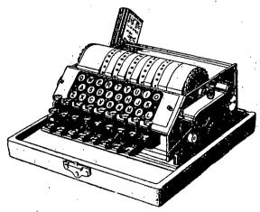
FIG. 10.-ELECTRICAL CIPHER MACHINE EMPLOYING A TYPEWRITER KEY-BOARD
