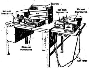
FIG. 12 .-- A PRINTING TELEGRAPH CIPHER MACHINE
